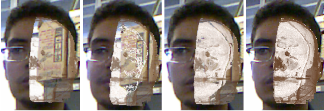
Figure 4.19 Influence of the parameter w_{grayLevel} in visible background on CT data. (a) w_{grayLevel} = 0 . (b) w_{grayLevel} = 0.5 (c) w_{grayLevel} = 0.75 . (d) w_{grayLevel} = 1 .
